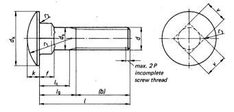
Designation of a mushroom head square neck bolt, with screw thread d=M 10, length l=70 mm and strength category 3.6 or 4.6 (at manufacturer's discretion):
